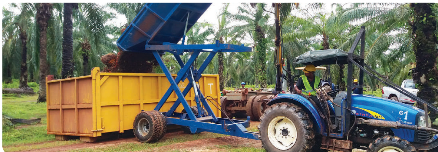
IOI implemented the mechanised FFB main line evacuation system using grabber in combination with bin transport system in about 40% of all estates across Peninsular Malaysia, Sabah and Indonesia.
