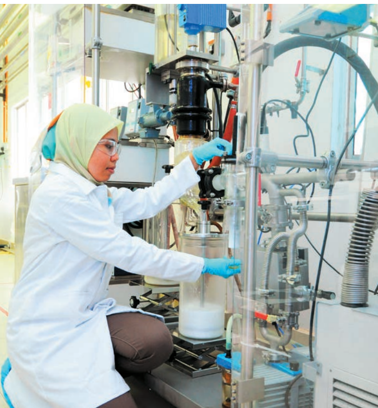
Thermal separation technique at IOI Loders Crocklaan Asia is conducted in meticulous care to separate oil into fractions and remove impurities based on specific temperature and vacuum.
